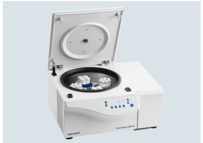
Centrifuge 5804 R with rotor S-4-72 (4 x 250 mL)
