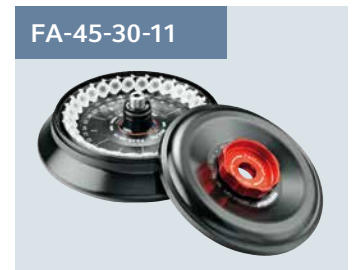
FA-45-30-11 30 x 1.5/2 mL micro tube rotor with aerosol-tight lid for safe centrifugation of hazardous samples. Max. speed 20,800 x g (14,000 rpm).
